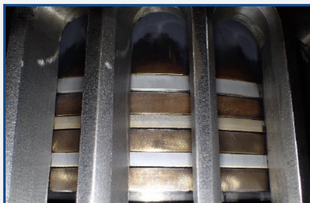
Unit 4: Infineum M7095 + Infineum Performance Booster
