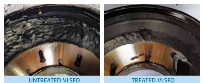
Images show low treat rate additive effect translated into real world performance in ship purifier systems
