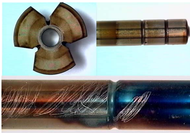
Figure 1: Armature plate, valve piston and nozzle needle with deposits consisting of polymeric organic material with additive related constituents. The scratches derive from a needle used to remove material for analysis.
