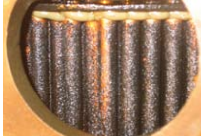
Gas engines in landfill service are susceptible to copper sulphide deposits on the oil cooler and hard silica deposits on the intake and exhaust valves
