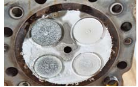
Gas engines in landfill service are susceptible to copper sulphide deposits on the oil cooler and hard silica deposits on the intake and exhaust valves
